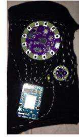
Fig. 1. Lilypad, ADXL Accelerometer and WiFi Module wired together using conductive thread to create smart wristband
